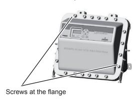
Fig. 7-11: X-STREAM X2 Field Housings and X2FD - How to Open
